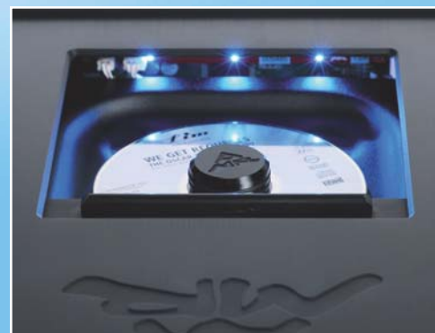
Three blue LEDs are designed to improve reading of the silver disks because the red laser operates at the opposite end of the spectrum (shown)
